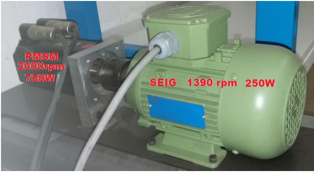
Figure 2: SEIG and PMSM motor is coupled to each others
